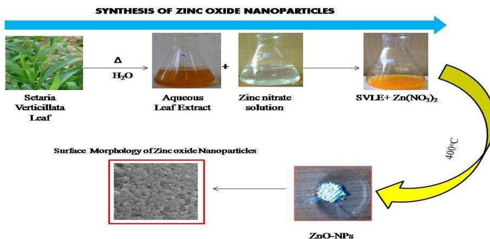
Figure4.1 Schematic synthetic croute of Zincoxide nanoparticles
